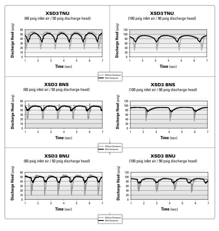
These charts show discharge head fluctuations for a diaphragm pump with and without a dampener. By reviewing the variation in pressure, the level of dampening can be estimated for an application. For example (XSD3 BNU 100/90), the head pressure generated by a 3" pump operating at 100 psig air inlet pressure and 90 psig head pressure varies between 30 psig and 94 psig resulting
