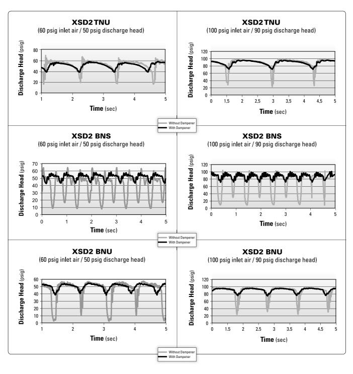
These charts show discharge head fluctuations for a diaphragm pump with and without a dampener. By reviewing the variation in pressure, the level of dampening can be estimated for an application. For example (XSD2 BNS 100/90), the head pressure generated by a 2" pump operating at 100 psig air inlet pressure and 90 psig head pressure varies between 6 psig and 102 psig resulting
