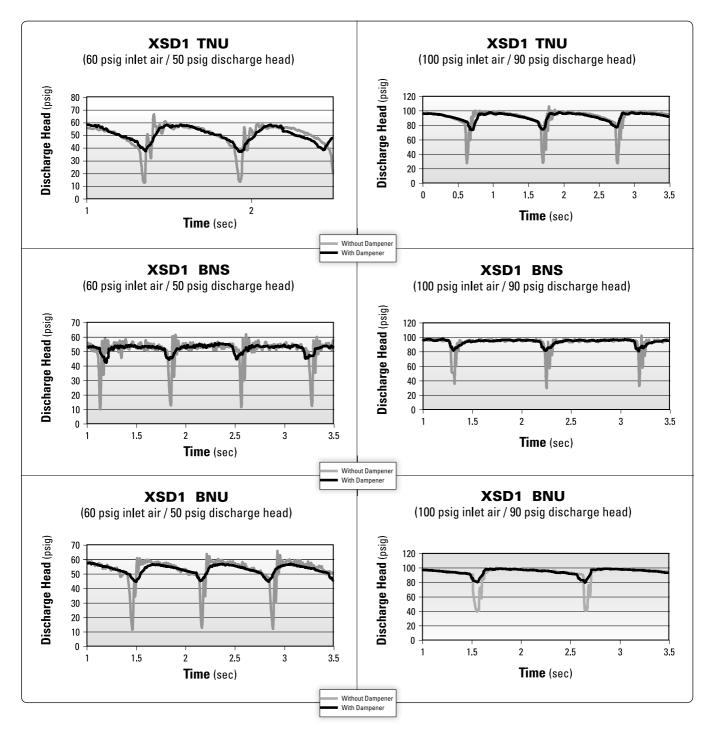
These charts show discharge head fluctuations for a diaphragm pump with and without a dampener. By reviewing the variation in pressure, the level of dampening can be estimated for an application. For example, the head pressure generated by a 1" pump operating at 100 psig air inlet pressure and 90 psig head pressure varies between 25
