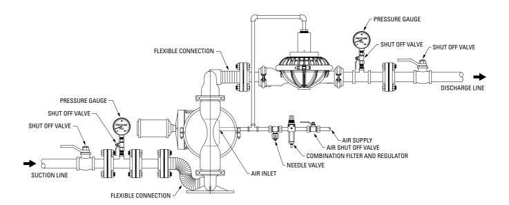
**NOTE**: In the event of a power failure, the shut off valve should be closed, if the restarting of the pump is not desirable once power is regained.
