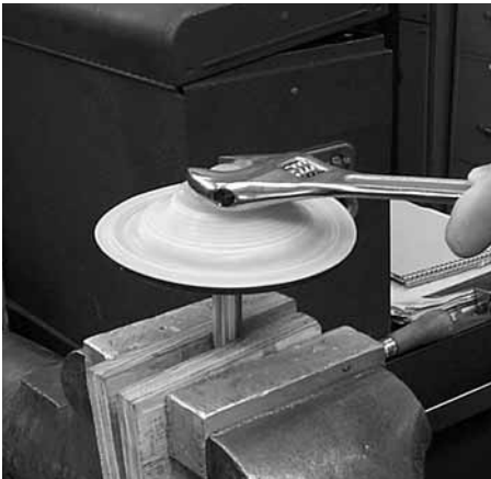
Step 11. Figure 11 To remove the remaining diaphragm assembly from the shaft, secure shaft with soft jaws (a vise fitted with plywood or other suitable material) to ensure shaft is not nicked, scratched, or gouged. Using an adjustable wrench, remove diaphragm assembly from shaft. Inspect all parts for wear and replace with genuine Wilden parts if necessary.
